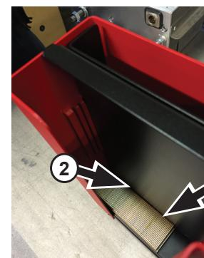
In the correct position, some space (②) remains between the staples and the black plate after loading staples in the compartment.
